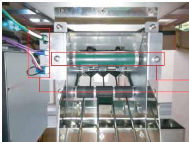
\* The adjustment of belt tension of FRA shall be made only when conveyor is not moving although FRA motor is normally working.
