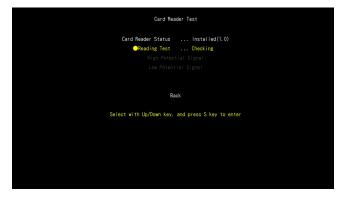
The status of card reader will show if the card reader is correctly installed, and card-reading status will show whether the reading is completed or fails.
