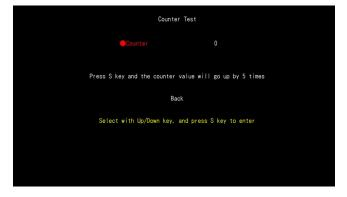
You cannot discontinue the counting process. When the counter is running, pressing the **S** button is useless.
