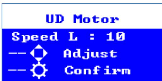
※ All motor speeds can be selected from 1-10, and the larger the number, the faster the crane moves
