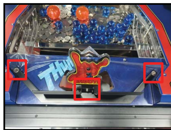
[ 1 ~ 2P ] SHOOTER ASS'Y PACKING BKT_2EA - Bolt, 6 Points *Replace with the supplied TH[M4x10L, 6EA] bolt.
