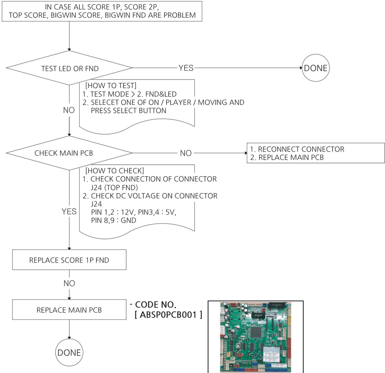
\* General check up : Check the supply voltage and wiring connection properly
