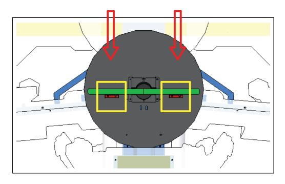
[ 1 ~ 2P ] BALL LIFT SCREW LED FAN STOPPER BKT\_2EA - Bolt, 4 Points
